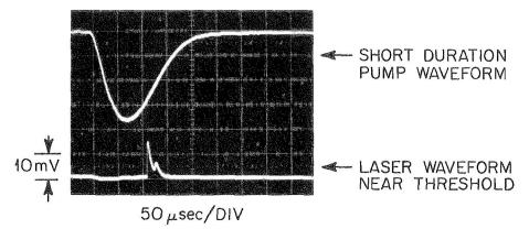
Fig. 3 Er:YAG laser waveform near threshold.
