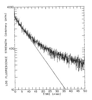
FIG. 2. Log of fluorescence signal decay vs time for the 1.06- $\mu$ m emission from the Nd<sup>3+4</sup>F<sub>3/2</sub> level in (10% Ho, 1% Nd):YAG.
