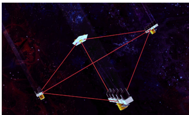
Fig. 1. A tetrahedral arrangement of separated spacecraft for very long distance interferometry. The spacecraft are locked together by motion measurement and feedback.
