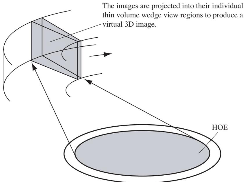
Fig. 5. The HOE/scene generator combination results in an individual image box.
