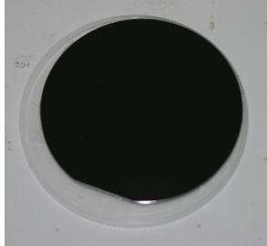
Fig. 2-1. Preliminary photodetector wafer.
