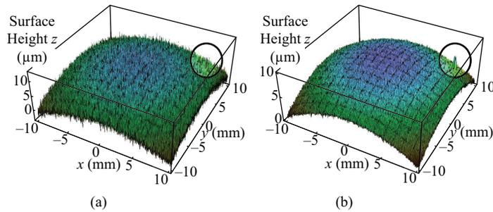
**Figure 1.** Metrological measurements have some unavoidable noise, which can hide small surface features (a). Some of these features can be recaptured through the use of statistical noise reduction (b). The feature is in the circled area on these graphs.
