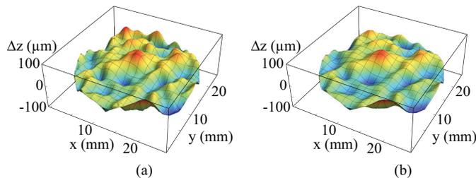
**Figure 2.** We reduced the  $2\sigma$  delta deviation ( $\Delta z$ ) of a battered calibration sphere from a raw measurement value of  $\pm 36.8 \mu\text{m}$  (a) to  $\pm 31.6 \mu\text{m}$  (b)—within 1% of the actual value of  $\pm 31.2 \mu\text{m}$ —by applying statistical noise reduction.
