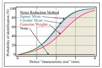
**Figure 3.** Probability of identifying a 3-µm feature with no noise reduction (black), Gaussian-weighted noise reduction (red), circular-mean noise reduction (green), and squaremean noise reduction (blue)
