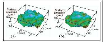
Figure 6. Surface deviation residuals before (a) and after (b) noise reduction
