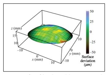
**Figure 7.** Surface of the sphere with locations measured from its center; surface color shows deviation from nominal (after noise reduction)
