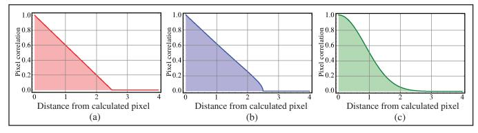
Figure 2. Correlation induced by statistical noise-reduction processes, shown assuming statistical range of 5 pixels for (a) square mean sampling, (b) circular mean sampling, and (c) Gaussian-weighted sampling
