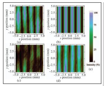
**Figure 8**. Noise reduction in interferometry: the original interferogram (a) was fit to a sinusoid with intensity varying from 0 to 1 (b); the difference between these two is the noise pattern (c); after noise reduction, the interferogram is much clearer (d); all follow the scale (e)
